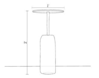
Material: Sand Casted Aluminium Finish: Matte Black Dimensions: l' (Diameter) x 2' (Height) Number of Components: l Weight: 5 kgs
