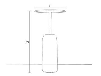
Material: Sand Casted Brass Finish: Buffed Brass Dimensions: l' (Diameter) x 2' (Height) Number of Components: l Weight: 22 kgs
