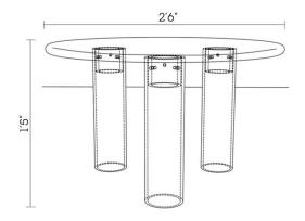
Material: Sand Casted Brass Finish: Buffed Brass Dimensions: 2'6" (Diameter) x l'5"(Height) Number of Components: 4 Weight: 70 kgs
