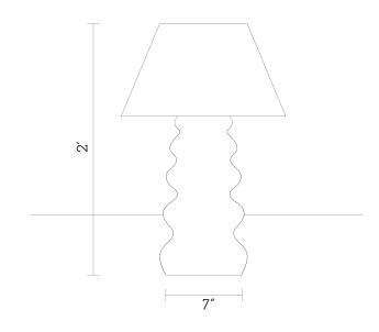
Material: Fiber Finish: Matte White Dimensions: Base: 7"(Diameter)x16"(Height) Shade: 8.5" (Top Diameter) 1'4" (Bottom Diameter) 9" (Height) Total Height: 24" Number of Components: 2
